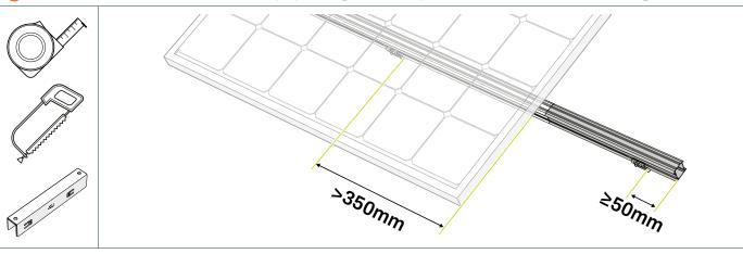
b. If the calculated overhang is less than 350mm beyond the marked position of the last seam clamp, keep 20-35mm rail length overhang for mounting the end cap (art. no. ) (>40mm for the ClickFit EVO 60mm clamp).
